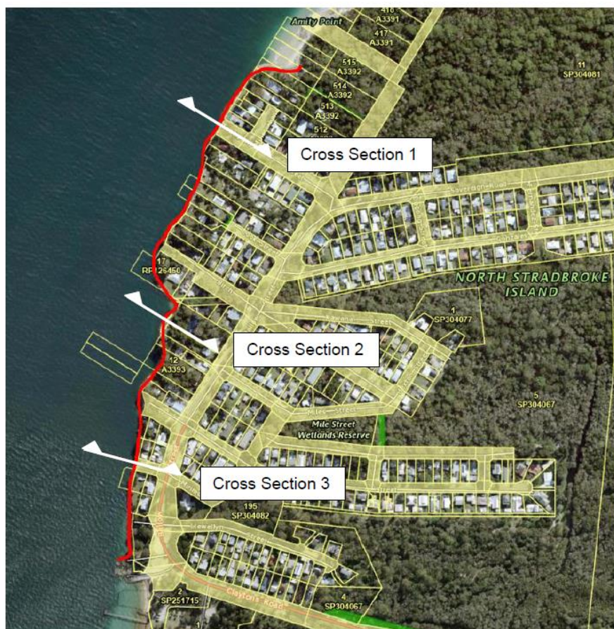
Figure 2-1 Extent of flow slide barrier and location of design drawing cross-sections
