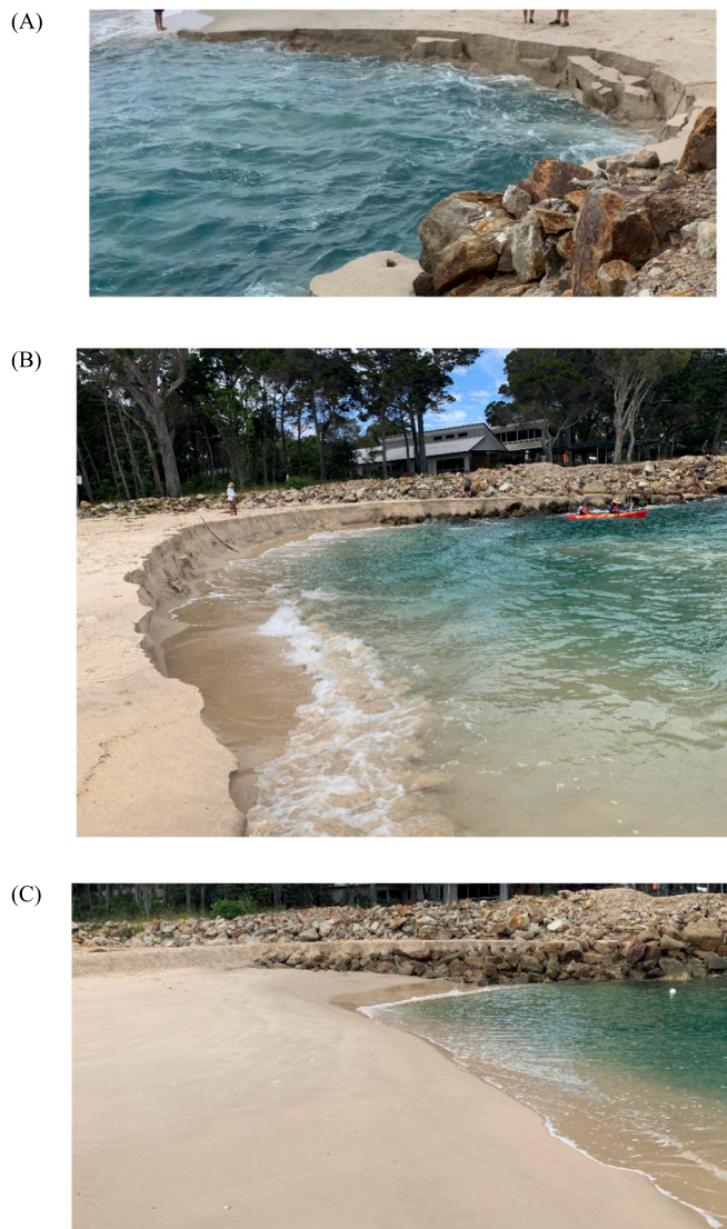
Fig. 2. (A) Propagating phase (B) termination phase (C) the recovery phase in a flow slide event recorded on 14/01/2023 at Amity Point field site.
