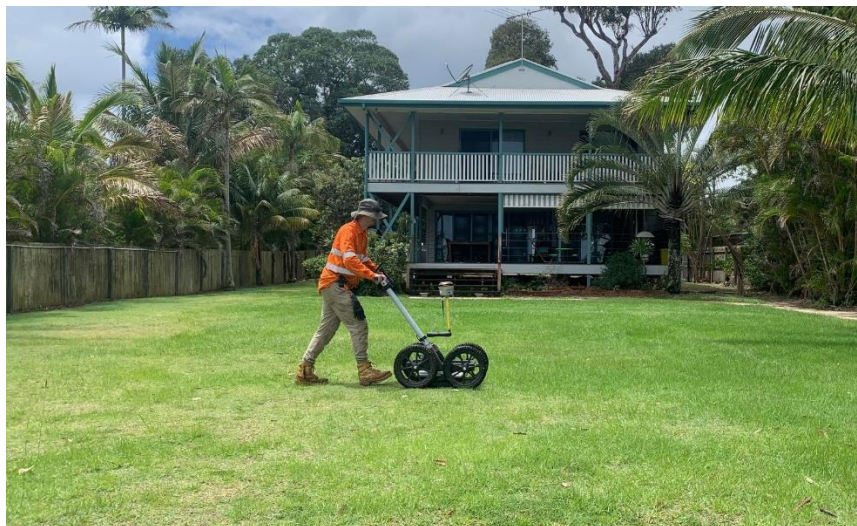
Inset 3: GPR survey underway in typical site conditions
