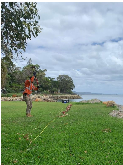
Inset 1: MASW streamer set-up on FSB, using sledge hammer seismic source
