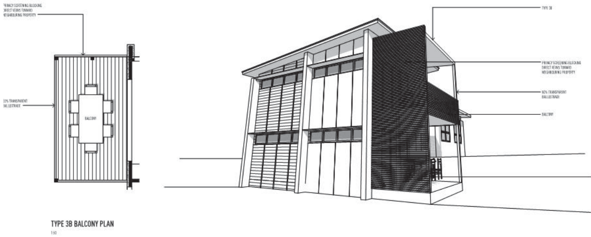
Figure 6. Detail design of window and privacy screen.
