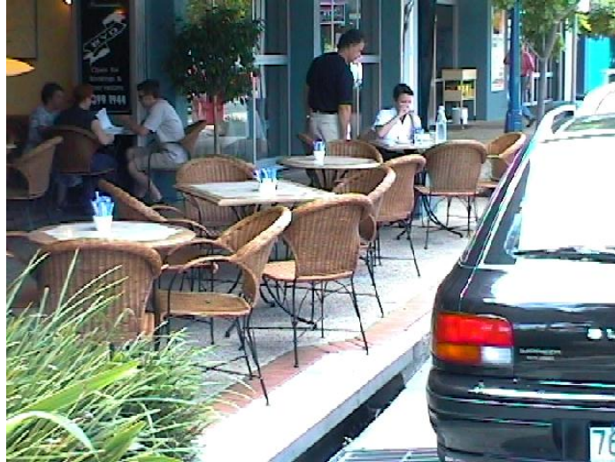
Photograph 5 - Insufficient separation to kerb
