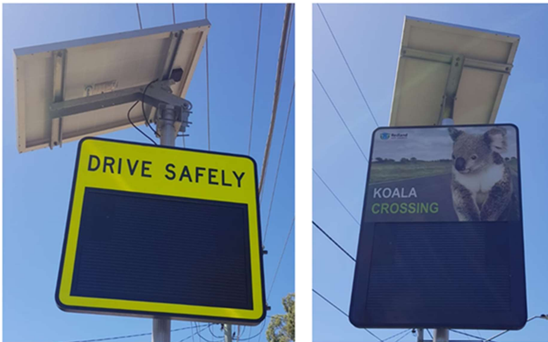
Figure 1. Sierzega brand models of dynamic (variable) message signage, named for this project as Jenoptik 'generic smiley' (left) and 'koala smiley' (right).
