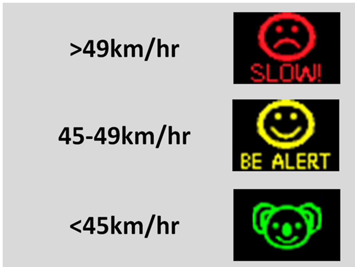
Figure 2. An example of the dynamic, variable sign messaging that greeted drivers given certain measured vehicle speed thresholds, capable with the Jenoptik models. In this example, messaging was tailored to a 50 km/hr posted speed limit zone. For a 60 km/hr posted speed limit zone, each threshold was increased by 10 km/hr. The green koala symbol
