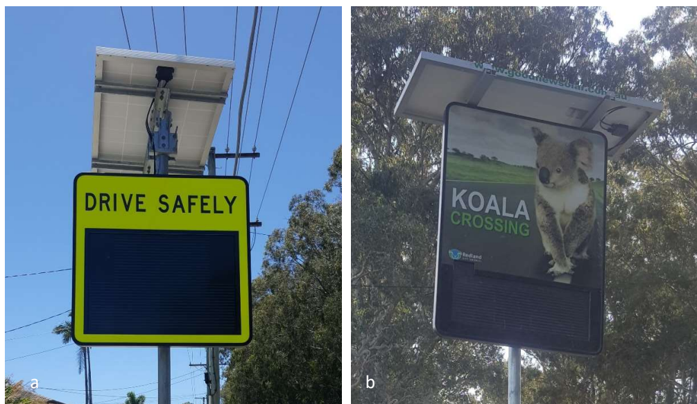
Figure 2. The signs used in the sign trial. a) a smiley sign, Sierzega Speedpacer 4568 C, and b) a koala sign, Sierzega Speedpacer 2368 FC.
