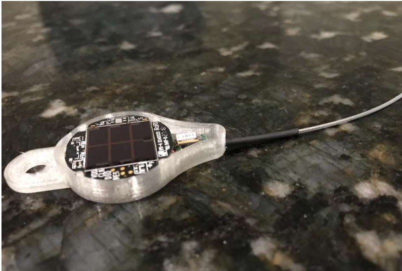
Figure 5 Version 5 (V5) solar Bluetooth tag is mounted in 3D print with some of the reinforced antenna protected in the casing so that in the occurrence of a breakage there is still some length of internal antenna and therefore some range
