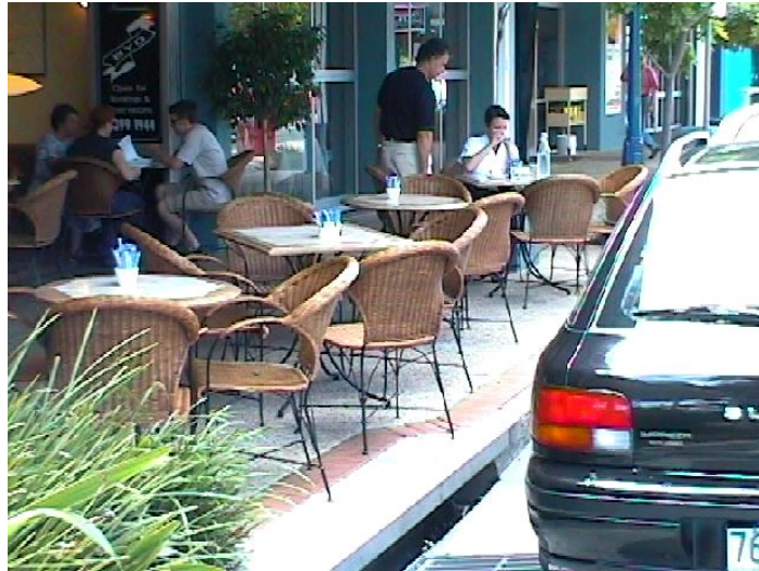
Photograph 5 - Insufficient separation to kerb
