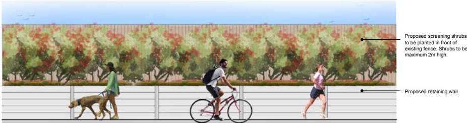
BETTER BY DESIGN: The footpath, retaining wall and planting design for the eastern side of Collins Road.
