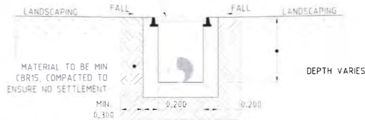
GRADED PIT DETAIL - LANDSCAPING SCALE 1:25
