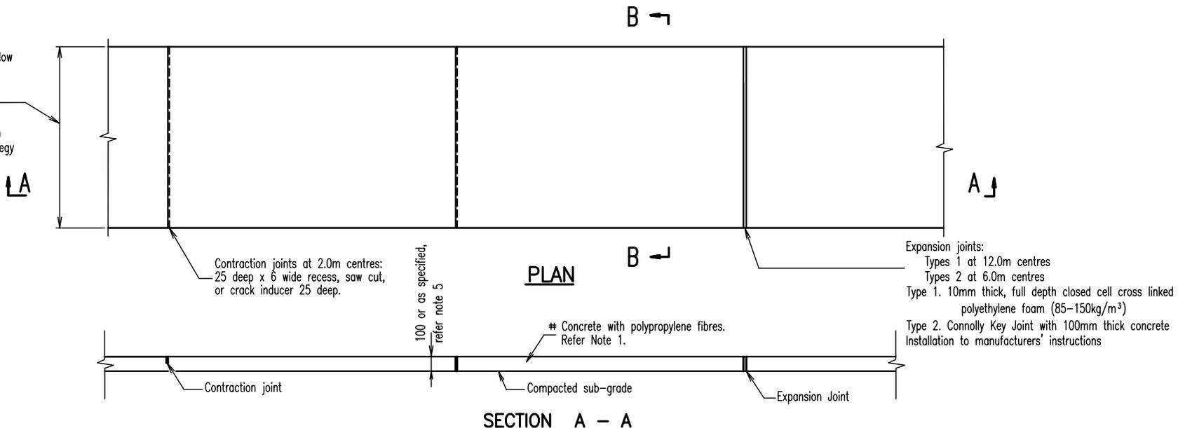
**FIBRE REINFORCED CONCRETE SPECIFICATION**
