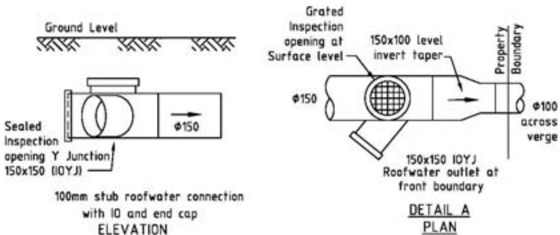
**ACCEPTABLE ROOFWATER DRAINAGE SYSTEM**
