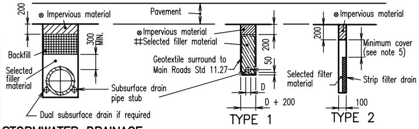
**STORMWATER DRAINAGE TRENCHES WITH SUBSURFACE DRAINAGE**
