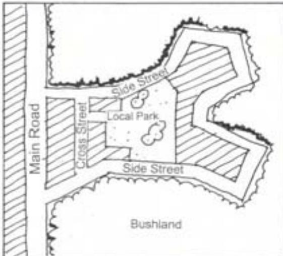
Acceptable – perimeter road system provides separation between hazard and assets; access for fire fighters, and provides two directions for evacuation.
