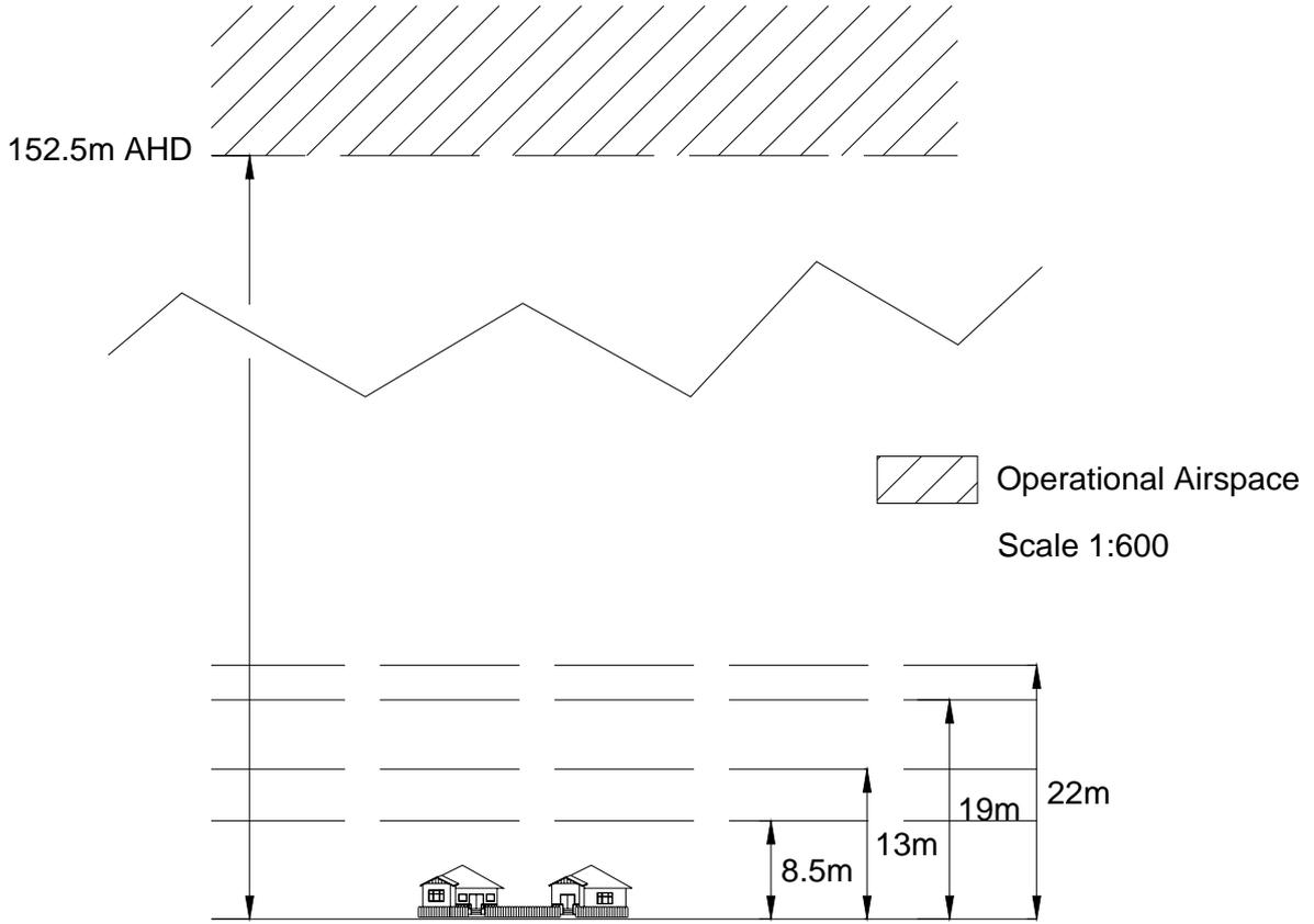
Diagram 2 - Areas affected by Mount Hardgrave Surveillance Radar Sensitive Area
