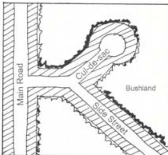
Unacceptable – closed road system congregates evacuation and response traffic, access for fire response restricted.
