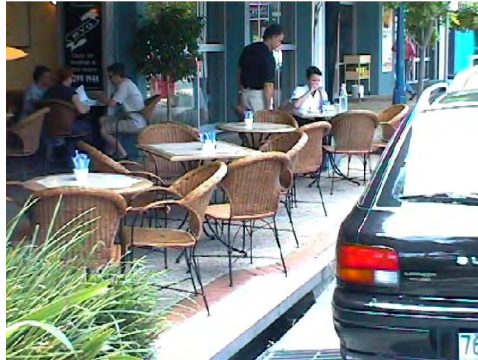
Photograph 5 - Insufficient separation to kerb
