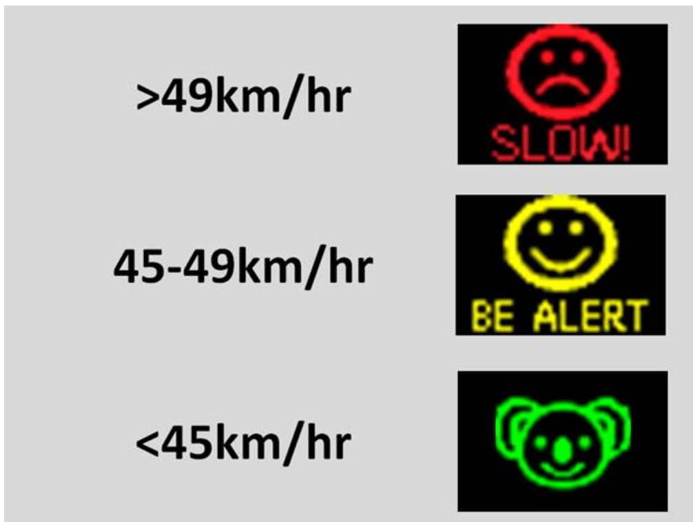
Figure 3. An example of the dynamic, variable sign messaging that greeted drivers given certain, measured vehicle speed thresholds, capable with the Jenoptik models. In this example, messaging was tailored to a 50km/hr posted speed limit zone. For a 60km/hr posted speed limit zone, each threshold was increased by 10km/hr. The green koala symbol which greeted drivers if they were recorded to be driving under 45km/hr (or under 55km/hr in a 60km/hr zone) was unique to the Jenoptik koala_smiley model (i.e. the generic Jenoptik smiley model featured a green, round ‘smiley’ face as pictured for the other speed thresholds).
