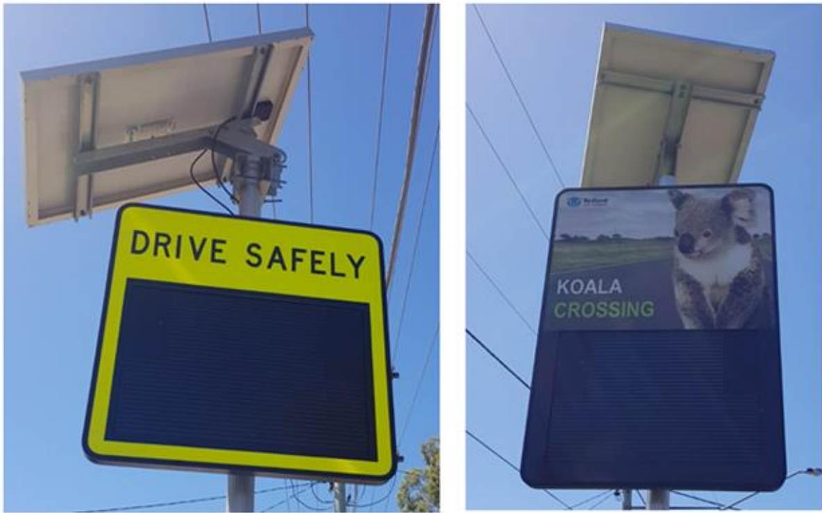
Figure 2. Jenoptik brand named for this project as ‘smiley’ (left) and ‘koala_smiley’ (right) models of dynamic (variable) message signage
