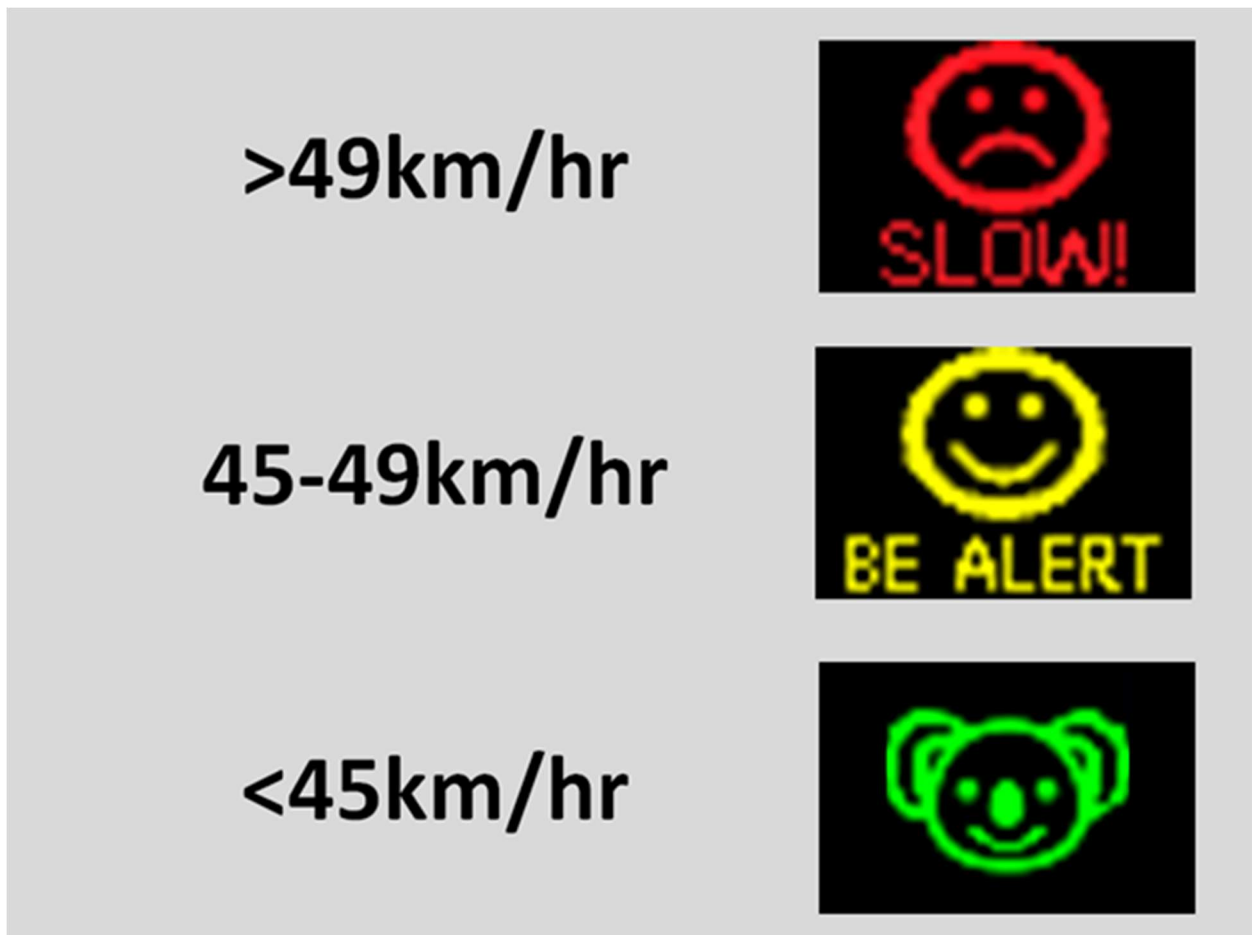
Figure 4. An example of the dynamic, variable sign messaging that greeted drivers given certain measured vehicle speed thresholds, capable with the Jenoptik models. In this example, messaging was tailored to a 50 km/hr posted speed limit zone. For a 60 km/hr posted speed limit zone, each threshold was increased by 10 km/hr. The green koala symbol that greeted drivers if they were recorded to be driving under 45 km/hr (or under 55 km/hr in a 60 km/hr zone) was unique to the Jenoptik koala smiley model (i.e. the generic Jenoptik smiley model featured a green, round 'smiley' face as pictured for the other speed thresholds).
