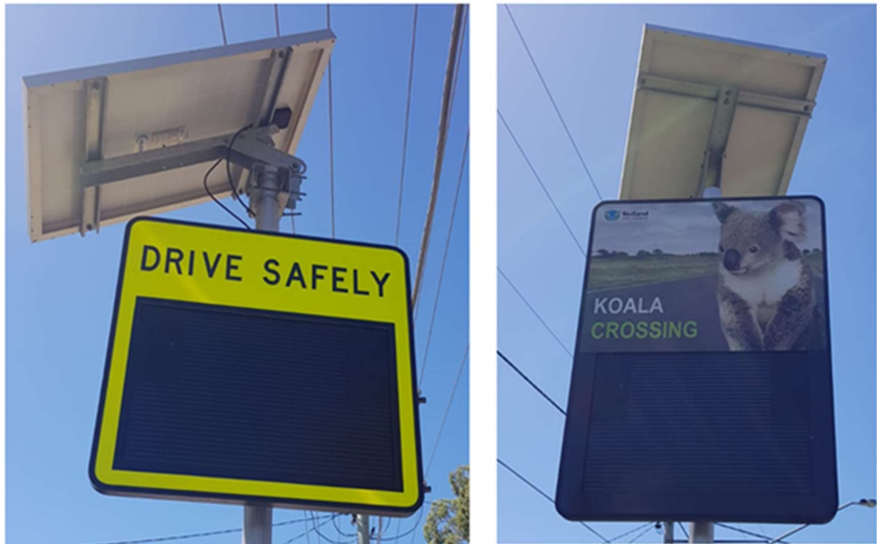
Figure 2. Sierzega brand models of dynamic (variable) message signage, named for this project as Jenoptik ‘smiley’ (left) and ‘koala smiley’ (right).
