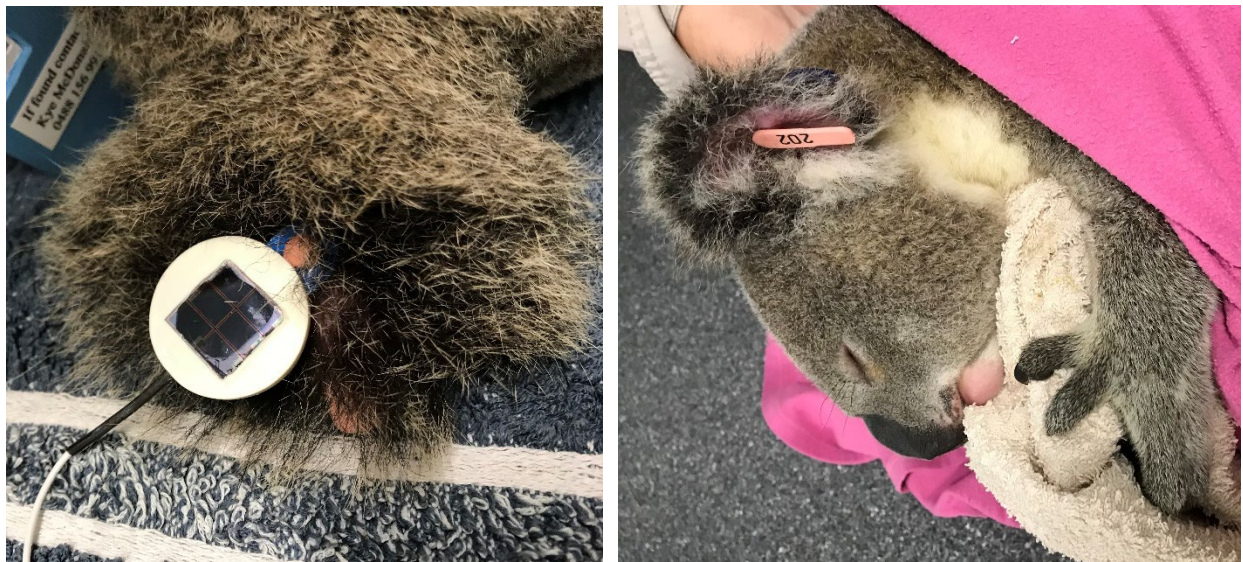
Figure 10 Bluetooth ear tags used during the second deployment as fitted on an Ormiston koala
