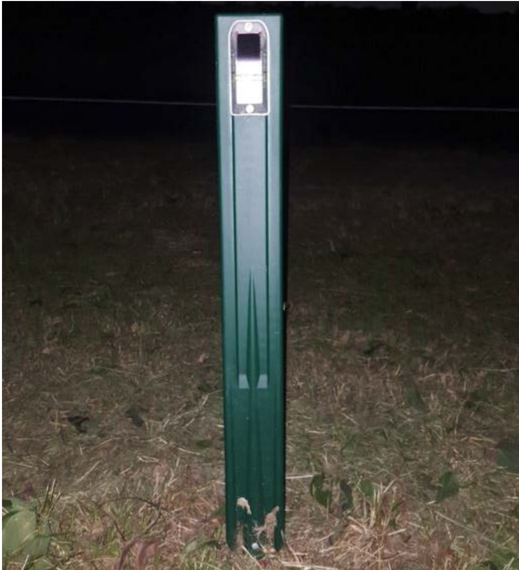
Figure 2. Virtual fence device in-situ on Heinemann Road showing device itself and a green, plastic installation post.
