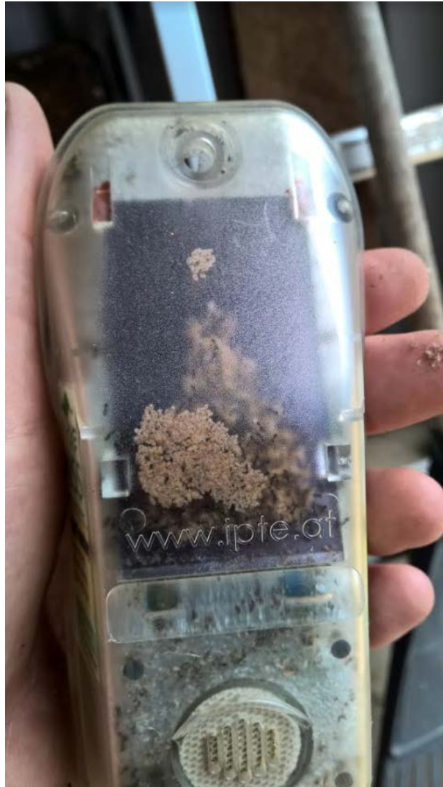
Figure 3. Ants infesting a VF device and subsequently requiring offsite repair/maintenance
