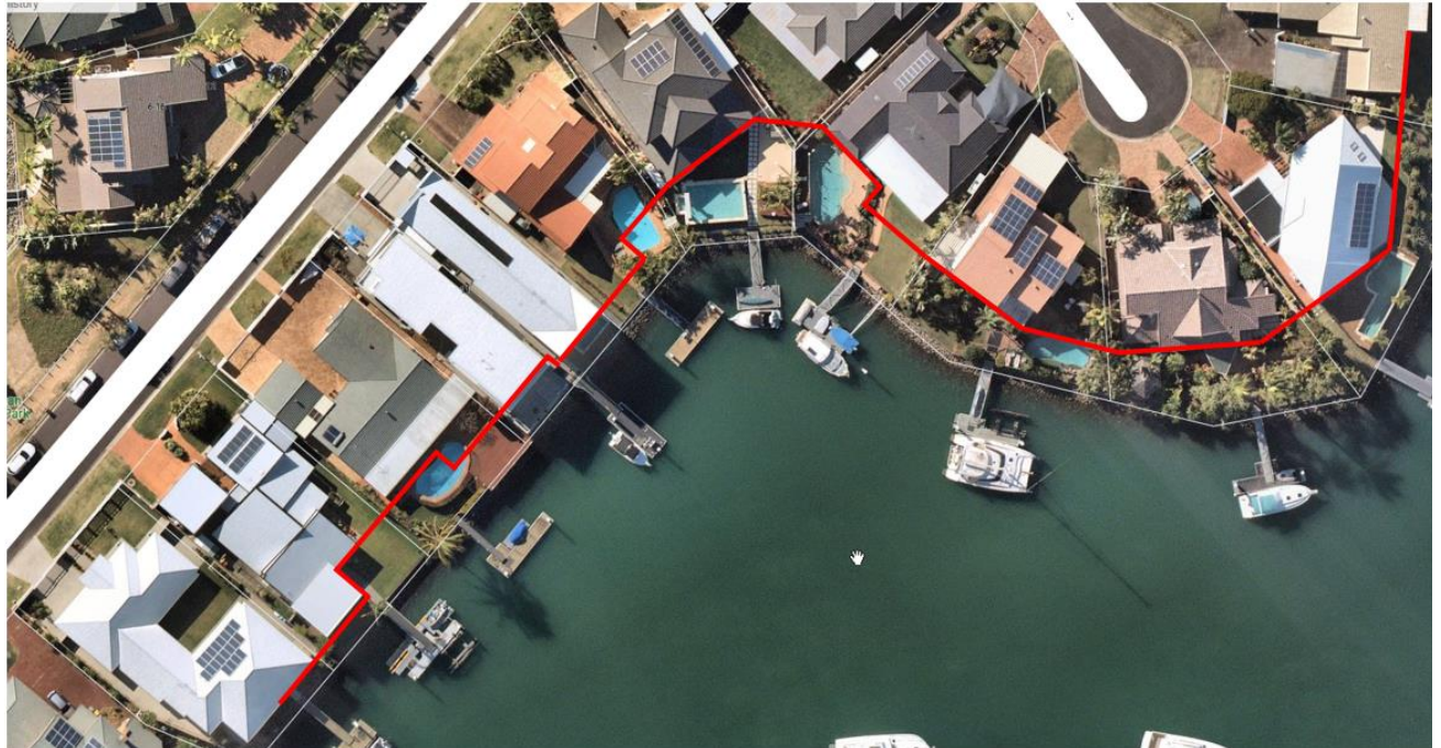
Figure 6.2.1.2.7 – To achieve compliance with PO9, dwellings may develop closer to the canal/lake, up to the red line. The centre of a site is used to delineate the location on the site where the red line changes to reflect the setback of the adjoining dwelling.
