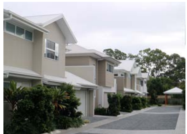
Parking integrated into the building design. Varied materials for access road punctuates and visually shortens the length of the access road. Change in materials can act as a traffic calming device
