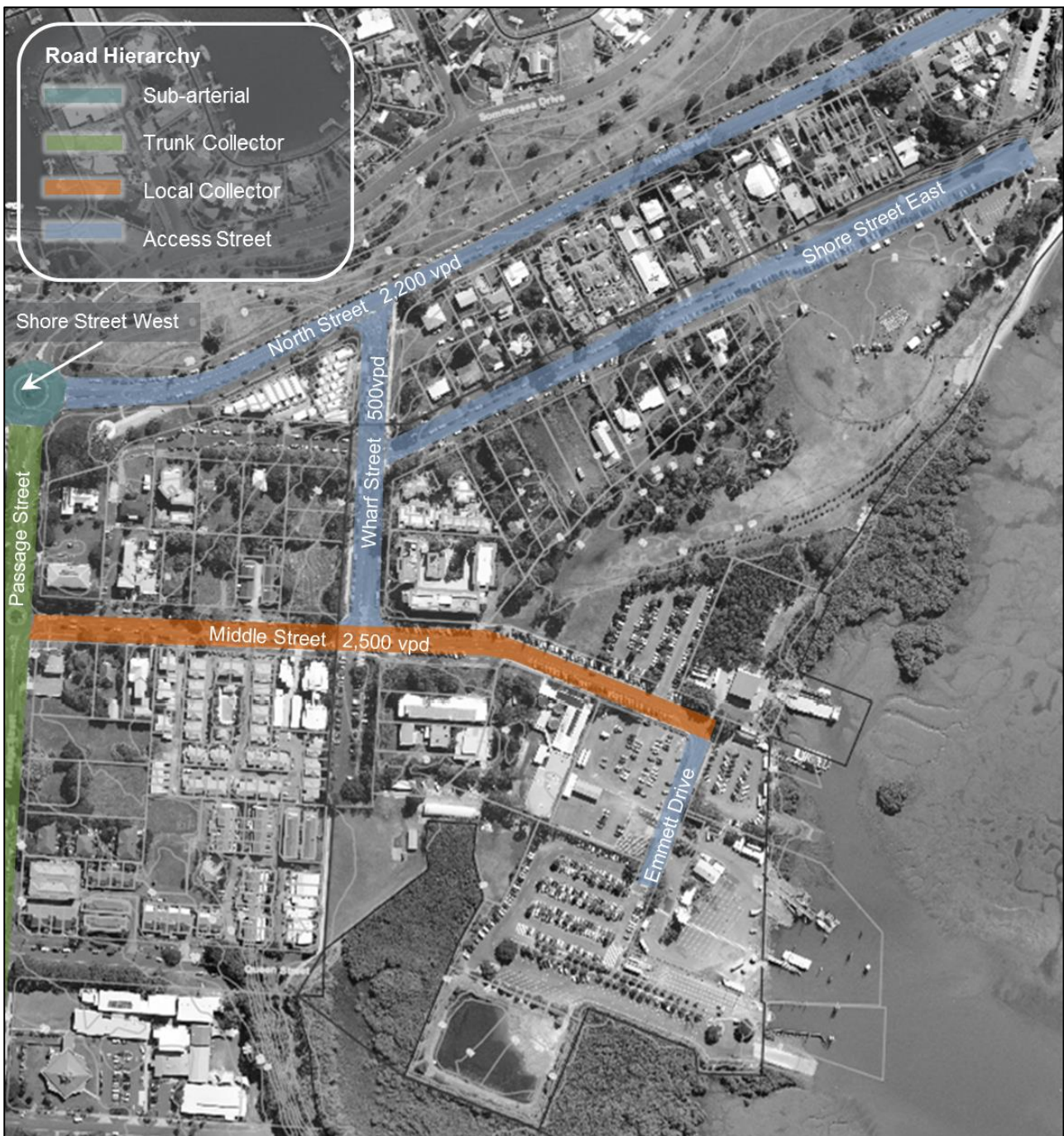
Figure 2-4 Existing Road Hierarchy and Traffic Volumes
