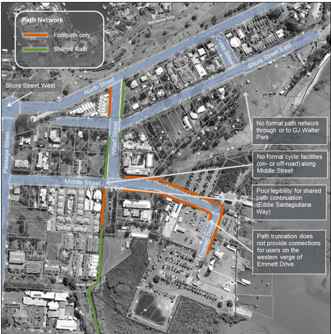
Figure 2-2 Existing Active Transport Network – Provision and Issues
