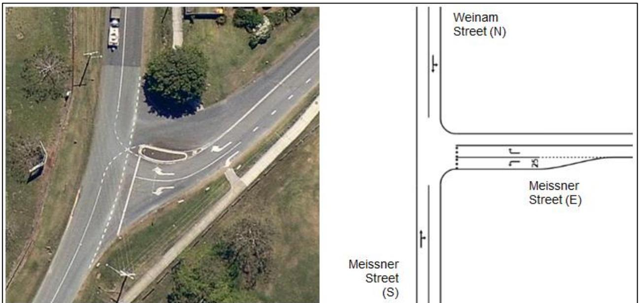
However, as the Priority Infrastructure Plan for Redland City has indicated a lane duplication for the corridor, this has been incorporated into the analysis as a future upgrade. Figure 6-7 illustrates the analysed intersection form. Analysis results have indicated that the upgraded form will be able to adequately accommodate future traffic demands without exceeding capacity thresholds.
