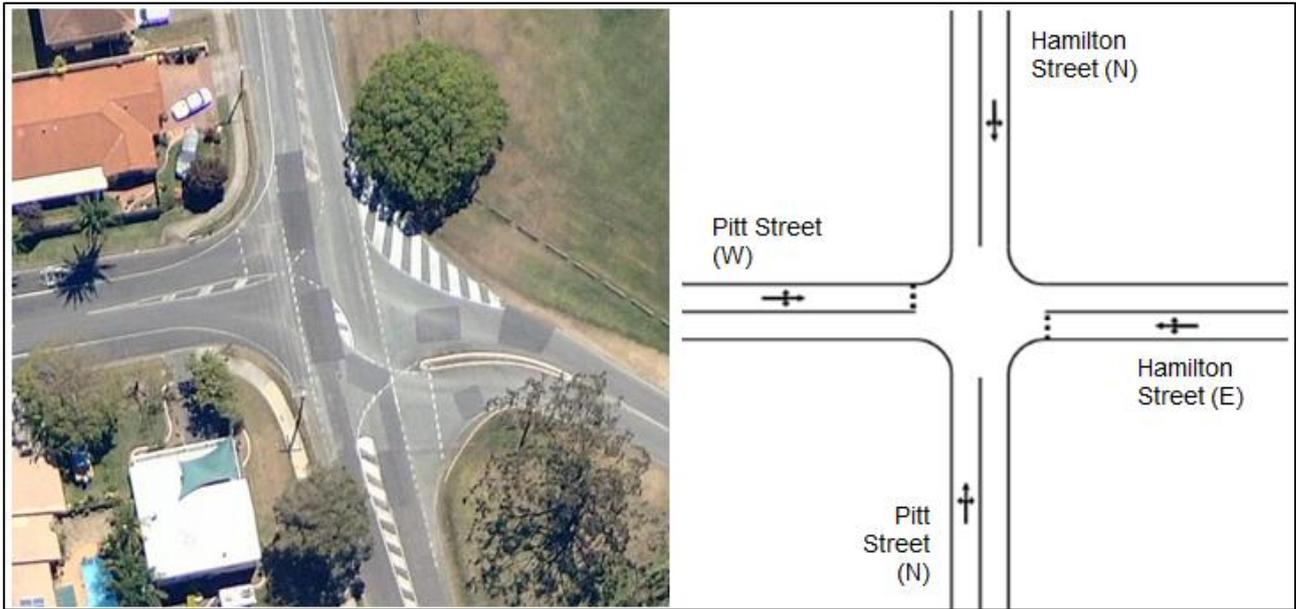
However, as the Priority Infrastructure Plan for Redland City has indicated a lane duplication for the corridor, this has been incorporated into the analysis as a future upgrade. Additionally, as the intersection is a key crossing point for all users to and from the development, particularly vehicles and pedestrians, it is proposed that a signalised form will be the safest option.
