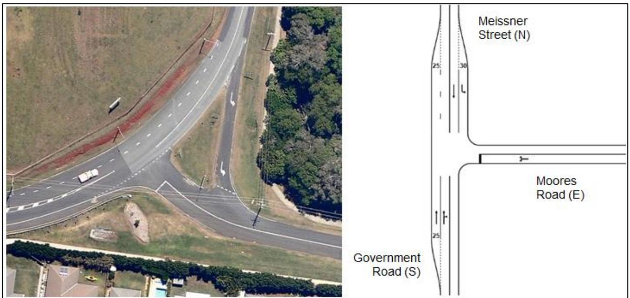
However, as the Priority Infrastructure Plan for Redland City has indicated a lane duplication for the corridor, this has been incorporated into the analysis as a future upgrade. Figure 6-9 illustrates the analysed intersection form. Analysis results have indicated that the upgraded form will be able to adequately accommodate future traffic demands without exceeding capacity thresholds
