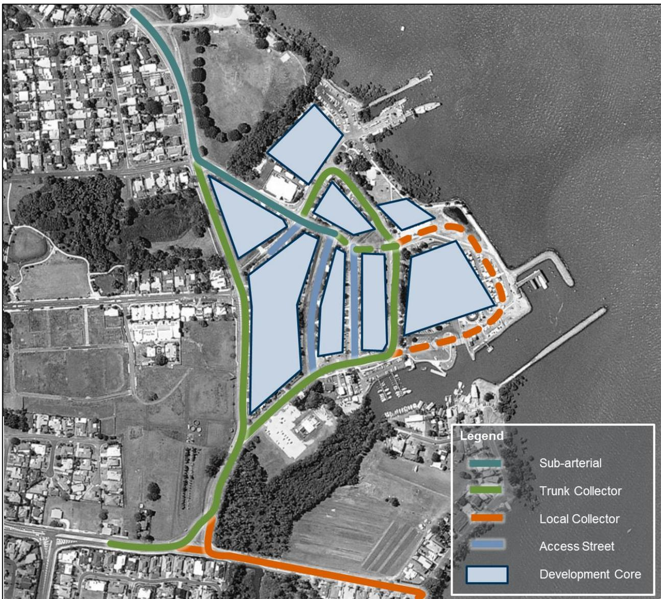
Table 4-2 describes the proposed road function with Table 4-3 summarising the road hierarchy of each of the study roads, while Figure 4-1 graphically illustrates the indicative road hierarchy of the structure plan.
